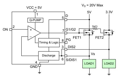
The highest  $V_D$  being switched must be at FET1 and pin 5 of the SLG55221 and SLG55220
