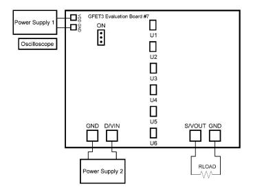
Figure 3. Typical connections for GFET3 Evaluation.
