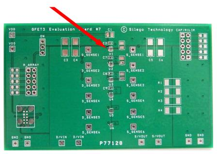
Figure 1. SLG59M307V Evaluation Board.
