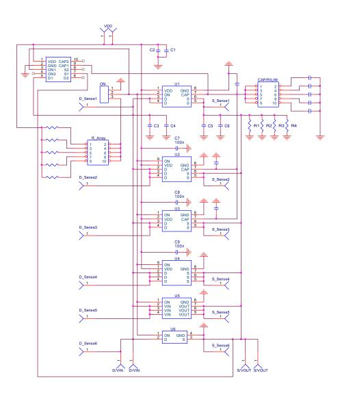
Figure 2. SLG59M307V Evaluation Board Connection Circuit.
