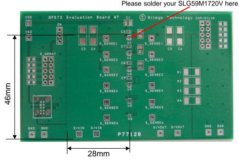
Figure 3. SLG59M1720V Evaluation Test Board
