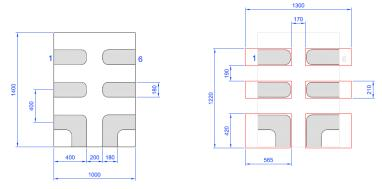
Figure 2. SLG59M1720V Package Dimensions and Recommended Land Pattern
