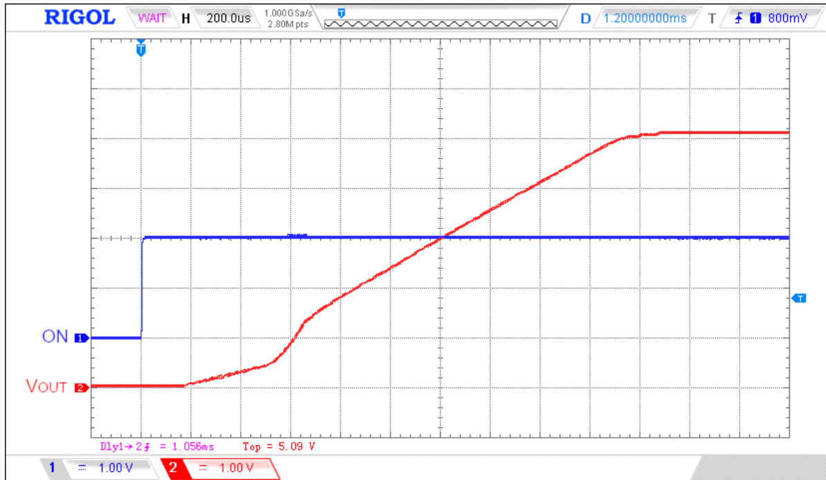
Figure 6. A SLG59M1717V with C_{SLEW} set to 4nF and 470μF for C_{LOAD} . C_{LOAD} -to- C_{SLEW} ratio is greater than 33,600. Note that the internal SCL monitor's been triggered and V_{OUT(SR)} is reduced until V_{OUT} reaches ~0.25V.
