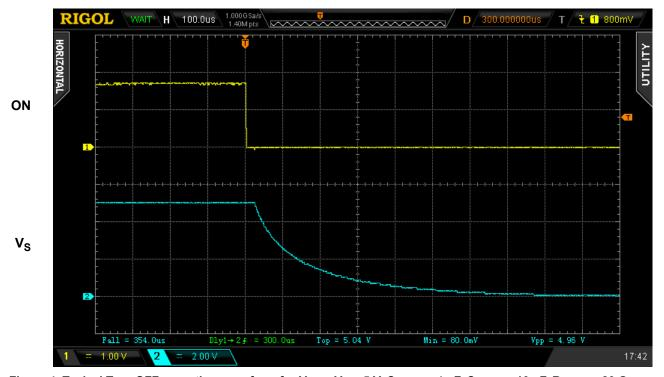
Figure 4. Typical Turn OFF operation waveform for V<sub>DD</sub> = V<sub>D</sub> = 5 V, C<sub>SLEW</sub> = 4 nF, C<sub>LOAD</sub> = 10  $\mu$ F, R<sub>LOAD</sub> = 20  $\Omega$
