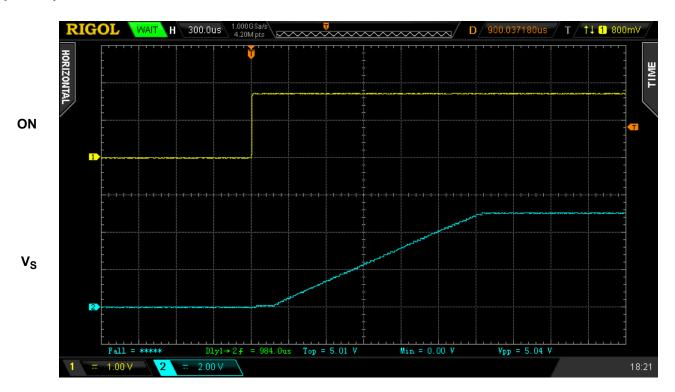
Figure 1. Typical Turn ON operation waveform for V<sub>DD</sub> = V<sub>D</sub> = 5 V, C<sub>SLEW</sub> = 4 nF, C<sub>LOAD</sub> = 10  $\mu$ F, R<sub>LOAD</sub> = 20  $\Omega$
