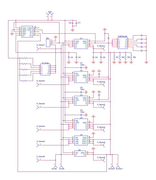
Figure 2. SLG59M1457V Evaluation Board Connection Circuit.
