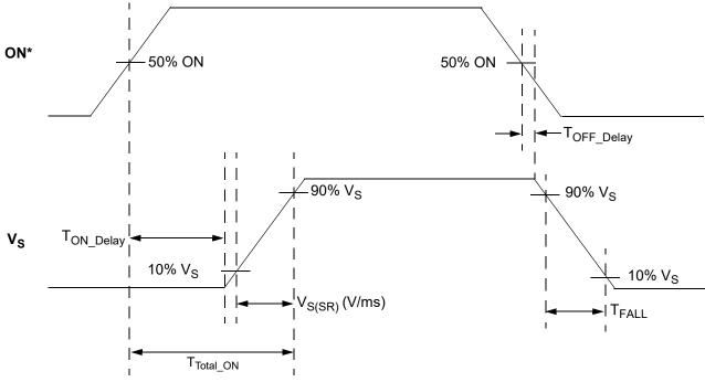
Note: \* Rise and Fall times of the ON signal are 100 ns
