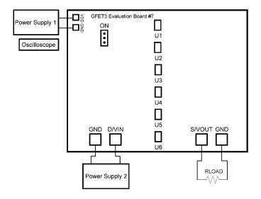
Figure 3. Typical connections for GFET3 Evaluation.
