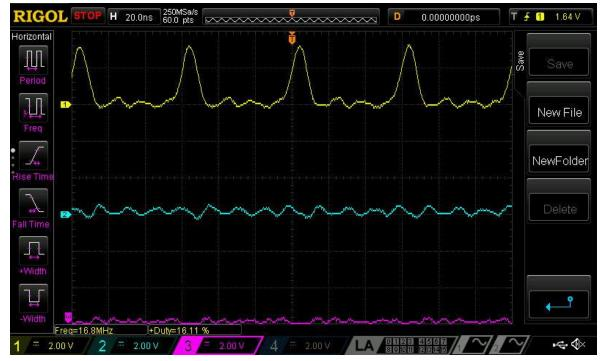
1. Period is 60ns. Pulse width is 10ns DC=16.7% (Correct functionality)
