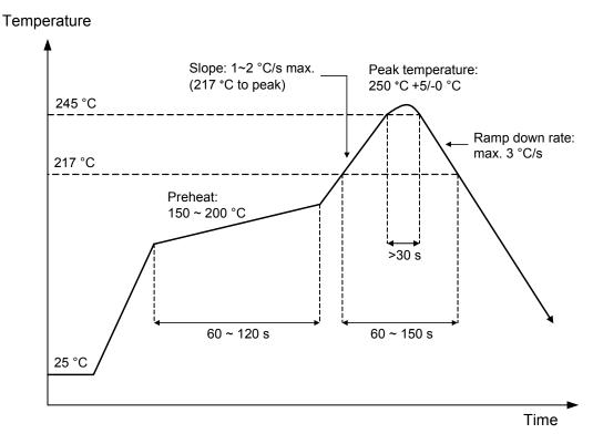
Figure 17: Reflow profile (lead-free)
