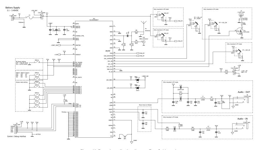
Figure 16 Example application diagram: Tour Guide mode
