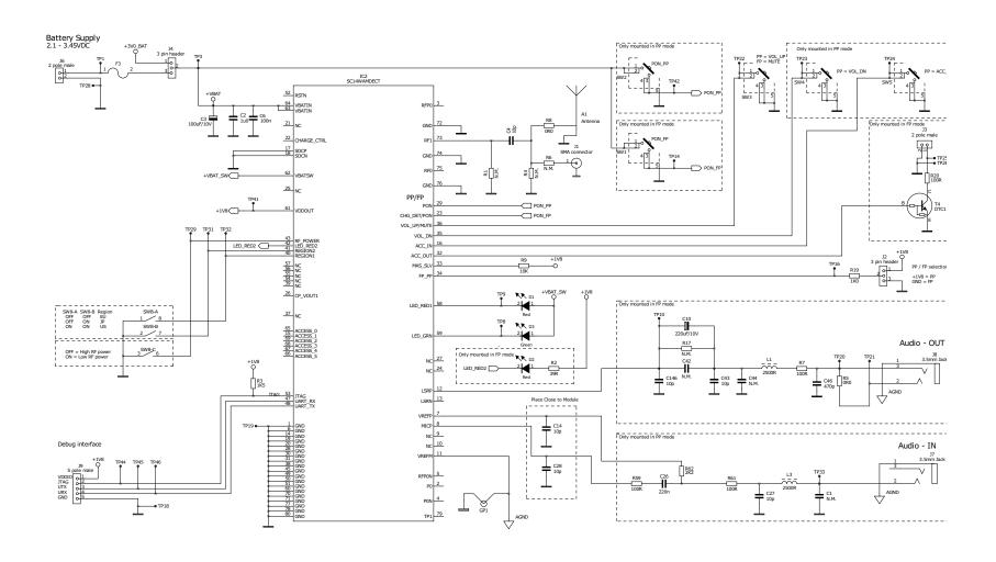
Figure 15: Example application diagram: Public Address mode
