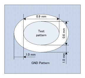
Figure 13: Clearance around test patterns
