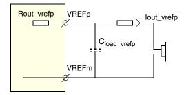
Figure 8: VREFp load circuit
