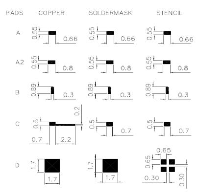
Figure 19: Copper pad, solder mask opening and stencil
