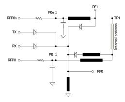
Figure 6: Internal circuit of the SC14WAMDECT SF
