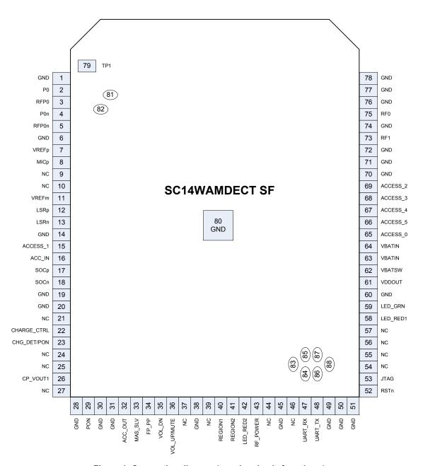
Figure 1: Connection diagram (top view, leads face down)
