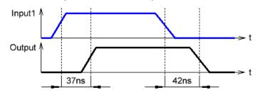
Figure 4: Serial Block Propagation Delay
