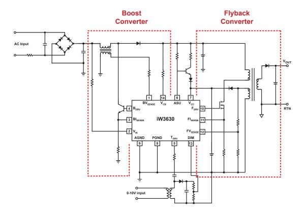
Figure 3.2: iW3630 0-10V Dimming Simplified Schematic
