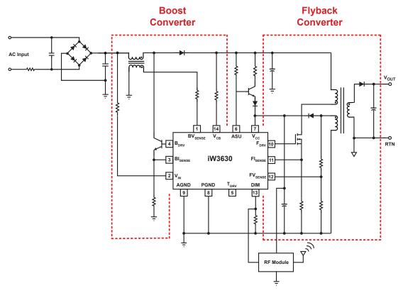
Figure 3.3: iW3630 Wireless Dimming Simplified Schematic
