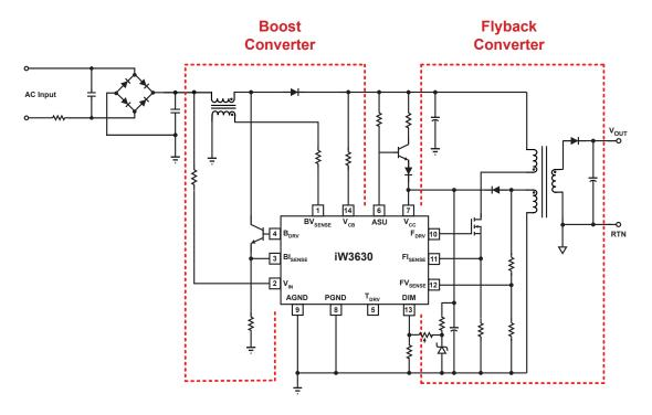
Figure 3.1: iW3630 Analog Dimming Simplified Schematic
