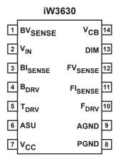
Figure 4.1: 14-Lead SOIC Package
