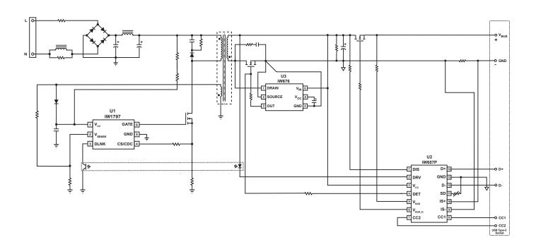
Figure 3.1 : iW1797 Typical Application Circuit for USB PD (Using iW657P as Secondary-Side Controller for USB PD and iW676 as Synchronous Rectifier Controller.)
