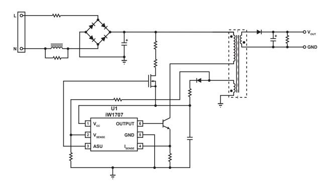
Figure 3.1 : iW1707 Typical Application Circuit (Using Depletion Mode NFET as Active Start-up Device)
