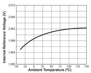
Figure 7.4: Internal Reference vs. Temperature
