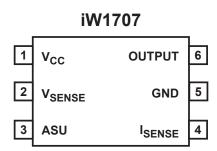
Figure 4.1 : 6 Lead SOT-23 Package
