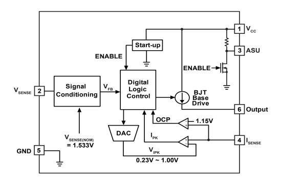
Figure 8.1: iW1707 Functional Block Diagram
