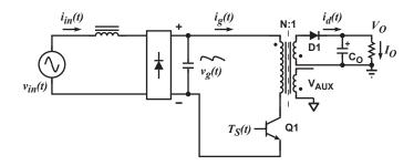
Figure 9.2 : Simplified Flyback Converter
