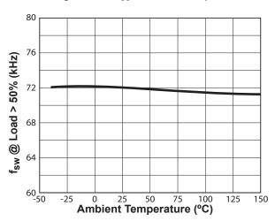
Figure 7.3 : Switching Frequency vs. Temperature<sup>1</sup>
