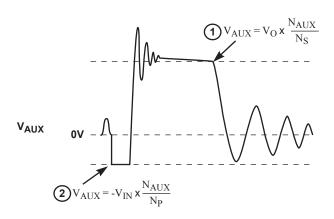
Figure 9.3 : Auxiliary Voltage Waveforms
