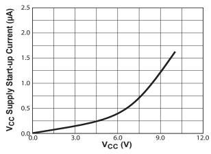
Figure 7.5 : V<sub>CC</sub> vs. V<sub>CC</sub> Supply Start-up Current
