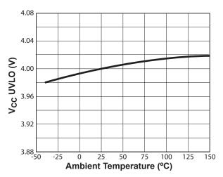
Figure 7.1 : V<sub>CC</sub> UVLO vs. Temperature
