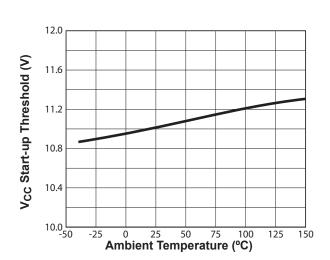
Figure 7.2 : Start-Up Threshold vs. Temperature
