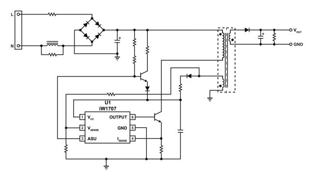
Figure 3.2: iW1707 Alternate Application Circuit (Using NPN BJT as Active Start-up Device)
