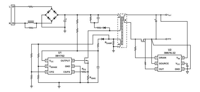
Figure 3.4 : iW1702 Typical Application Circuit with Supplement Output Over-Voltage Protection and iW676-32 Secondary Synchronous Rectifier Controller with Active Voltage Positioning.
