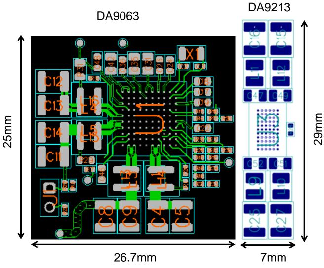
This layout example provides an indication of the area required for the ZU9 solution including the DA9063 and the DA9213. This example uses Automotive qualified components, the overall area could be further optimised if consumer grade parts were used.
