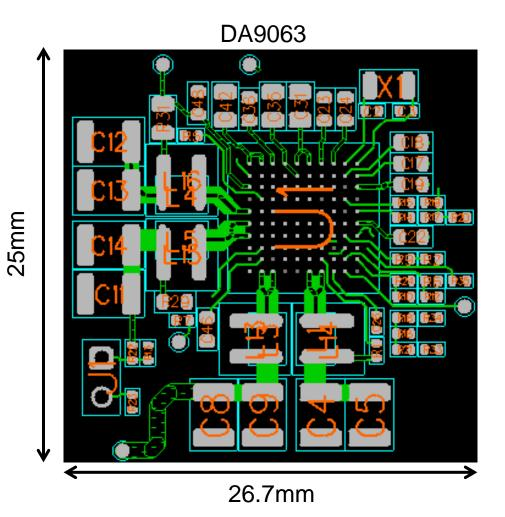
Note: in this layout the DA9063 has input decoupling in the reverse side of the board.
