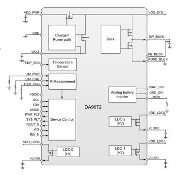
An integrated analog battery monitor facilitates on-demand battery voltage and discharge current monitoring for to create a battery fuel gauge solution. A watchdog input monitors the processor and upon detecting a stall in the processor, it power-cycles the buck converter to avoid an indefinite hang up in the system. Status outputs and I<sup>2</sup>C allow the host to set PMIC behavior and monitor its status.
