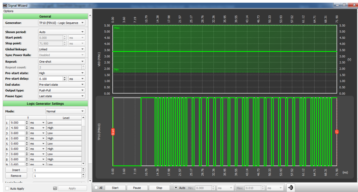
Figure 9: Signal Wizard Configuration on Pin10(IR-IN)
