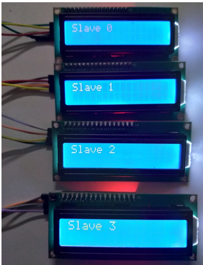
Figure 7: I 2 C-LCDs Outputs After Implementation
