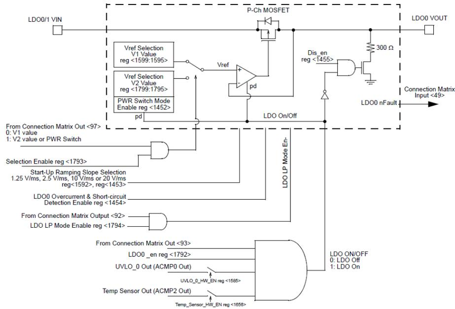
Figure 3: SLG46580 LDO0 Regulator Block Diagram
