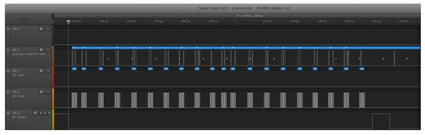
Figure 1: SPI transmitting device ID
