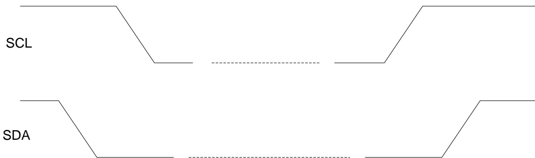
Figure 6: I 2 C START and STOP Condition Timing
