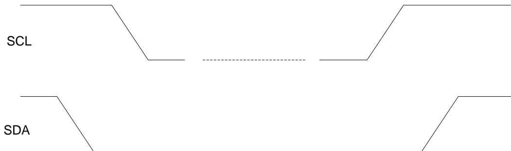
Figure 12: I 2 C START and STOP Condition Timing
