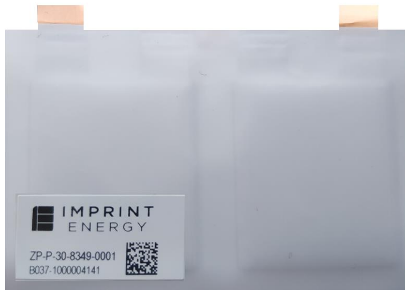
Figure 6: The actual 15mAh ZincPoly flex, ultra-thin battery
