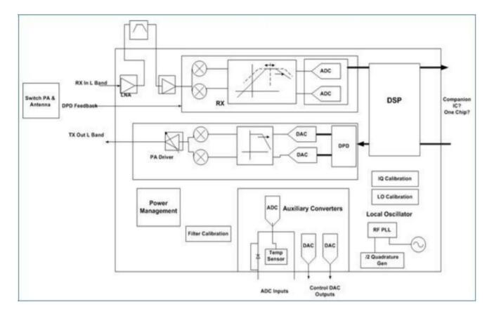
Figure 1: RF SoC Device Diagram
